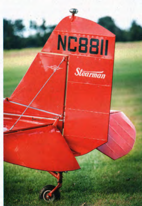
The entire aft section of the fuselage, including the tail had to be replaced with remanufactured C3B components.
