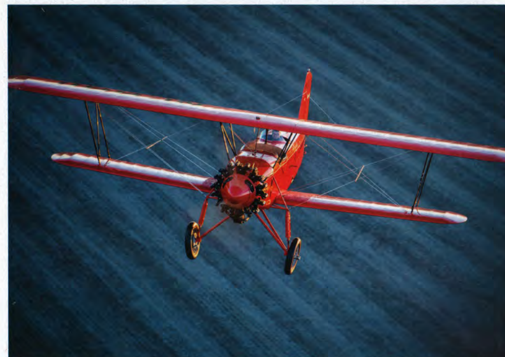
While the C3B and the C3R Stearmans appear to be similar airplanes, pilots report that the C3B's anachronistic and heavy control system was greatly improved in the C3R. The Kelch C3B also still uses the original J-5 Wright engine, which has some unique features, being a 1920s design. When not touring, the airplane is on display at the Kelch Aviation Museum in Brodhead, Wisconsin.
