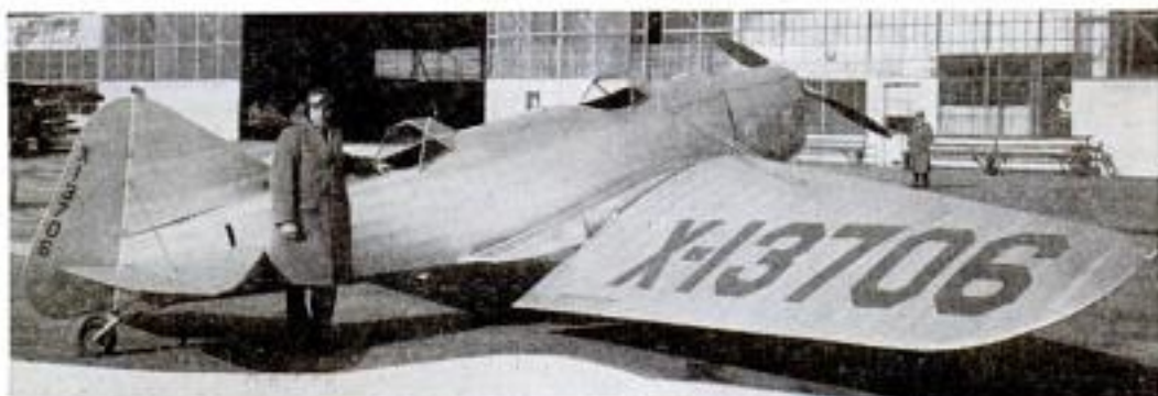
The Cornelius monoplane assembled and ready for flight. Notice that the outer wing is depressed below the stub, thus doing away with the necessity for ailerons.
